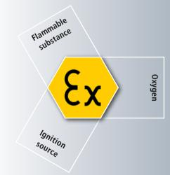
To prevent an explosion, one of the three explosion factors must be excluded. In most cases, this is the ignition source.
