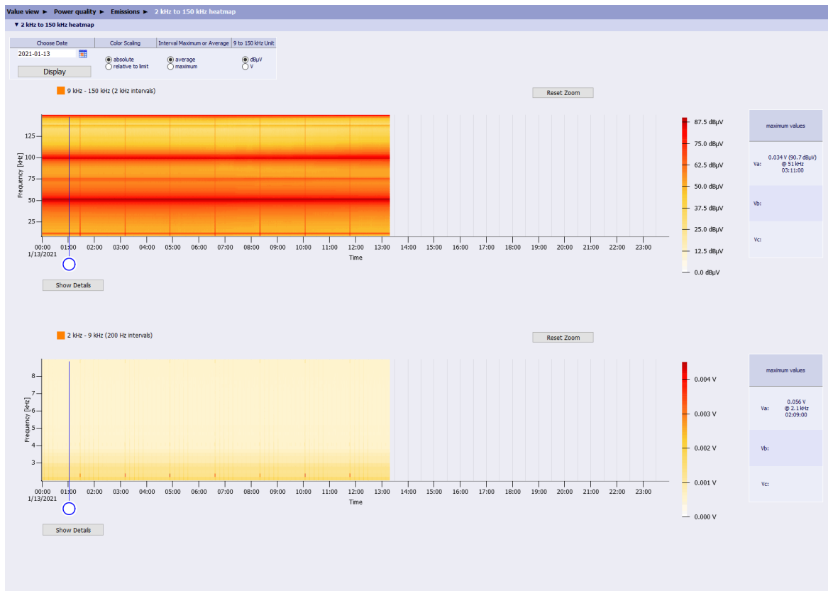
Figure 6-16 1-Day Record of the Emissions from 2 kHz to 9 kHz and from 9 kHz to 150 kHz; Average Values of the Magnitude
