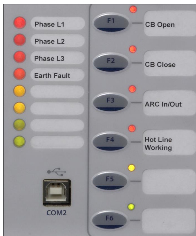
Fig1. Tri-colour LED's and function keys
