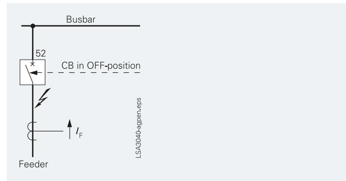
Fig. 10/8 End-fault between circuit-breaker and current transformer
