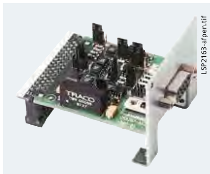
Fig. 11/13 RS232/RS485 Electrical communication module
