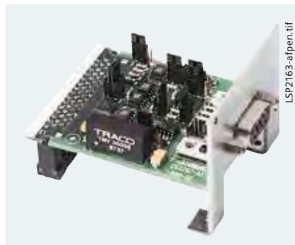
Fig. 6/22 RS232/RS485 electrical communication module
