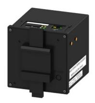
SENTRON, meas. device & power quality recorder, 7KM PAC5200, standard rail housing w/o display L-L: 690 V, L-N: 400 V, 10 A, strd rail instr., 3- phase, Modbus TCP, apparent/ Active/reactive energy / cos phi, harmonics: 2. - 40., THD, class 0.5 acc. to IEC61557-12 or cl. 0.5S acc. to IEC62053-22, wide-range pwr sup. unit AC/DC, screw terminals
