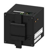
SENTRON, measuring device, 7KM PAC5100, strd mount. rail encl. w/o display, L-L: 690 V, L-N: 400 V, 10 A, strd rail instr., 3-phase, Modbus TCP, apparent /active/reactive energy / cos phi, harmonics: 2. - 40., THD, class 0.5 acc. to IEC61557-12 or cl. 0.5S acc. to IEC62053-22, wide-range pwr sup. unit AC/DC, screw terminals
