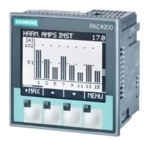
SENTRON, measuring device, 7KM PAC4200, LCD, L-L: 690 V, L-N: 400 V, 5 A, 3-phase, Modbus TCP, optional Modbus RTU / PROFINET / PROFIBUS / DI/DO, apparent/active/reactive energy / cos phi, harmonics: 2.-64., THD, class 0.2 acc. to IEC61557-12 or cl. 0.2S acc. to IEC62053-22, wide-range pwr sup. unit AC/DC, screw terminals
