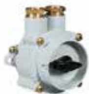
UNAV 2162 rotary two-way switch sockets in marine grey painted brass with UNAV 1948 cable glands 250V IP66
