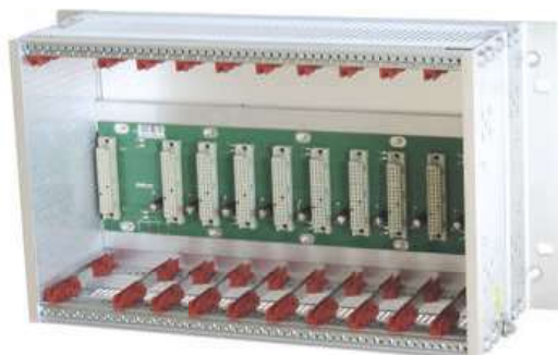
Example of chassis for 10 cards with bus backplane
