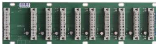
Example of RTU7M bus backplane with 10 slots
