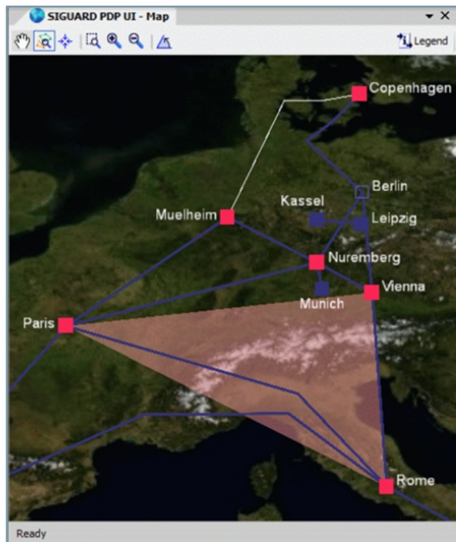
Figure 6.3/8 Visualization of a Detected Short-Circuit A Red Triangle Connects the 3 Stations Most Affected by the Short-Circuit
