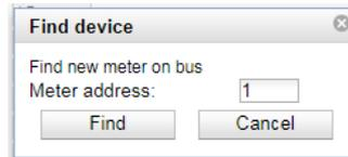
When the meter is found, a special query will automatically read all the over mentioned necessary information.
